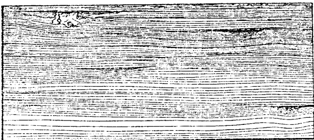
FIG. 1.—Longitudinal section of a board approximately quarter-sawn containing checks (radial section) (original).
